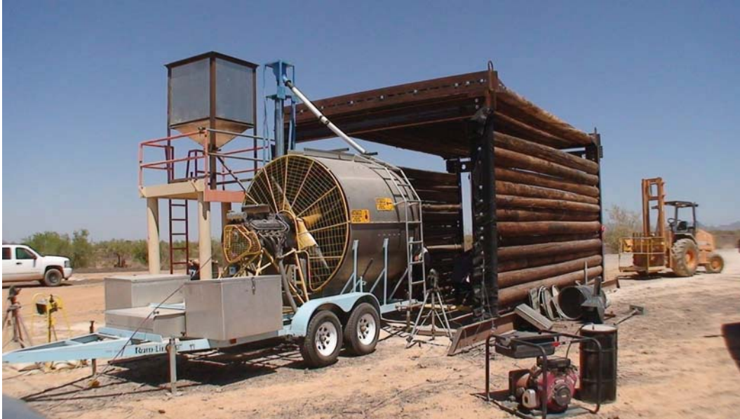
Figure 2. Typical Air Flow Straightener with 245 HP Wind Generator
